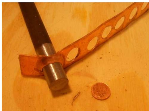
**Fig 2;** *deformation of the parent metal around the cold drill and the resultant punched disc*
