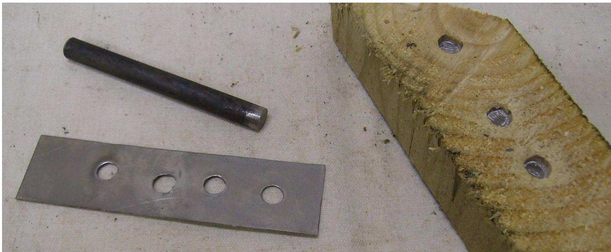
**Figure 3;** 6mm cold drill used on 1mm steel plate with the punched discs embedded in the end grain awaiting removal
